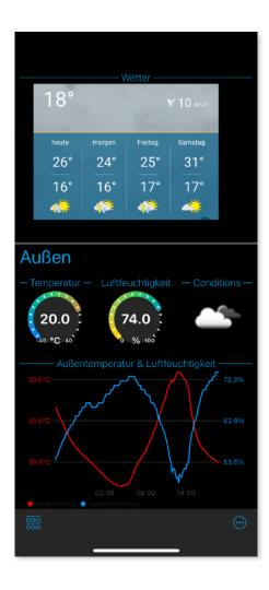
Visuals manages a so-called "Dashboard" which you can also see directly after the start of the app. The Dashboard is a scrolling list of widgets. A widget can be a pure display or an operating element such as a switch.
